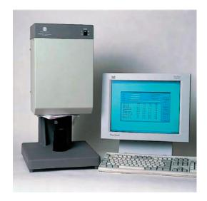
Highly competitive markets, such as the paper, pulp and cellulose industry, require a commitment to top quality throughout. With Konica Minolta's state-of-the-art Spectrophotometer CM-3630 and the accompanying PaperControl software you can precisely monitor production at all times.
